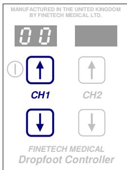
**Enter *Level Mode of Channel 1*** by pressing the two buttons on the left hand side of the *Controller* together simultaneously. The level will be shown on the corresponding displays. Use these **Up** and **Down** buttons to increase or decrease the value. Any changes in level are immediately reflected in the output.
