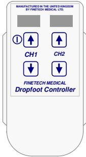
**The Controller** is the source of the power and signals that are transmitted to the *Implanted Receiver* through the skin by radio frequency inductive coupling. It is housed in a small plastic box with an integral rechargeable battery.
