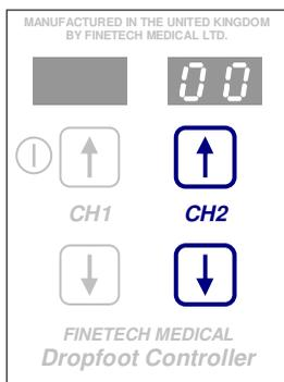
**Enter Level Mode of Channel 2** by pressing the two buttons on the right hand side of the *Controller* together simultaneously. The level will be shown on the corresponding displays. Use these **Up** and **Down** buttons to increase or decrease the value. Any changes in level are immediately reflected in the output.
