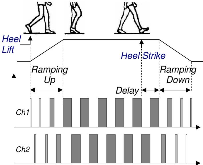
The *Controller* is activated from a *Footswitch* placed in the users' shoe. Stimulation begins when the heel is lifted off the ground. Stimulation is ended when the heel strikes the ground.
