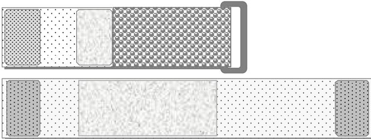
**The Footswitch** is used to detect heel-strike and heel-lift that triggers stimulation from the *Controller*. See [Section 4.1](#) for fitting instruction.
