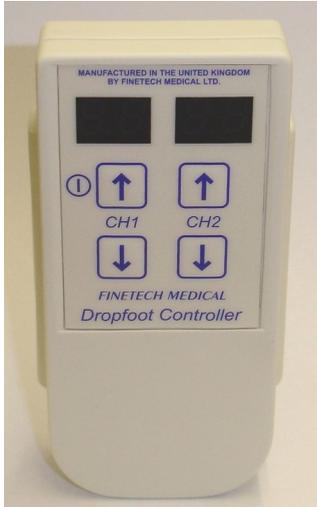
In order for the implant to receive correct stimulation the control box must be fixed in place directly over the implant. The implant is, typically, placed on the lateral aspect of the affected leg posterior and distal to the fibula head. To aid this placement the rear of the control box has a curved interface with a circular indent that is in-line with the internal transmitting circuit element.
