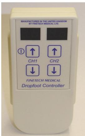
The Control Box is worn directly over the implant and transmits power and signals to the implant by radio frequency inductive coupling.
