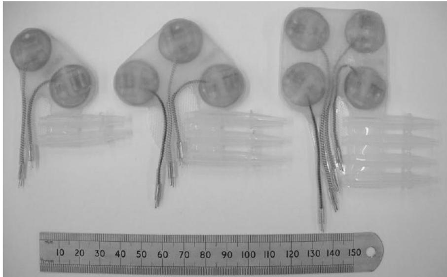
**Figure 5: 2, 3 and 4 Channel Receiver Blocks**
