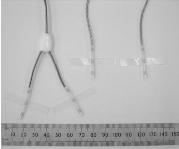
**Figure 7: Extradural Electrodes**
