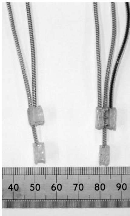
**Figure 6: 2 and 3 Channel Intrathecal Electrodes**
