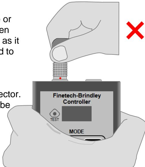
To unplug the connector from the *Transmitter Block*, hold the *Transmitter Block* in one hand and pull the metal part of the plug with the other hand.
