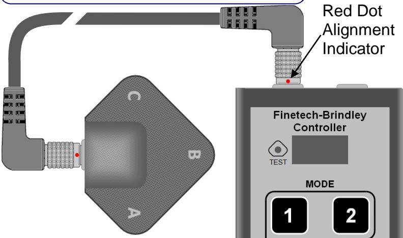
The connectors use a Push-Pull self-latching connection system, therefore the outer metal part of the connector is a moving part.
