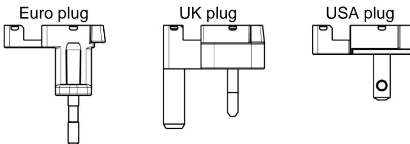
**Fitting a plug:** First align the plug with the fitting slots on the charger body, then push the plug into the slots and slide it forward until it clicks together.
