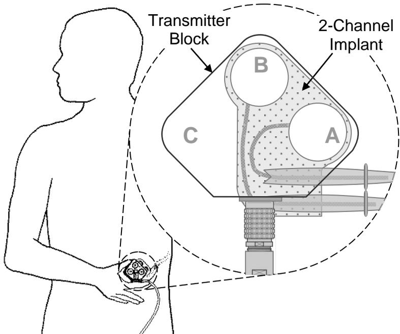
1. Place the *Transmitter Block* accurately over the *Receiver*.
