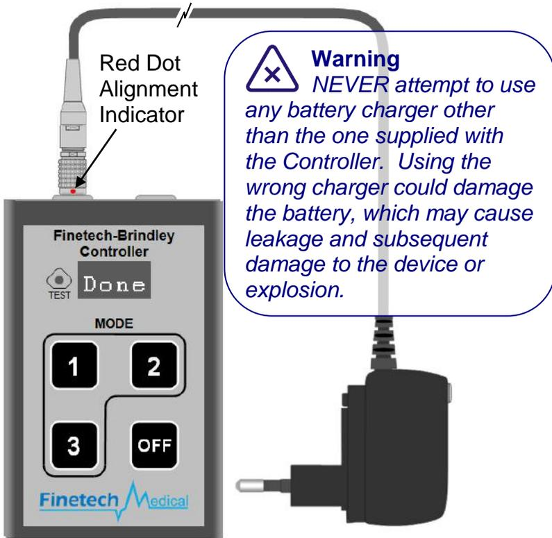
**When to charge:** The controller contains a Lithium-ion battery and can be charged at any time, whether at a 90% charge level or only 10%. Do not allow a nearly flat battery to be unused for more than a month or so; the battery will slowly discharge until it becomes fully
