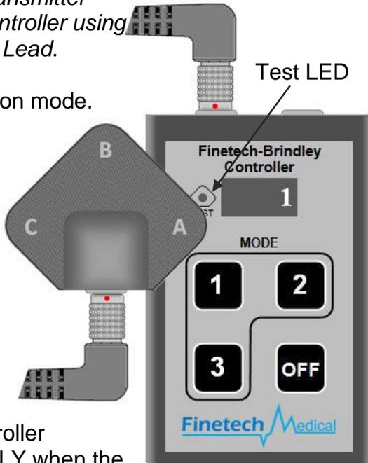
Note: The Controller transmitting ONLY when the mode number is flashing.
