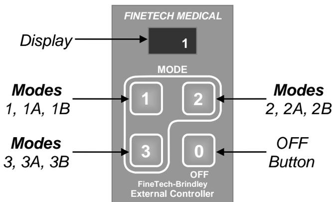
You select which Mode to use by pressing the corresponding Button. You cannot select a Mode which has not been set up for you. If you only use the stimulator for function 1, your clinician should have disabled Buttons **2** and **3**.
