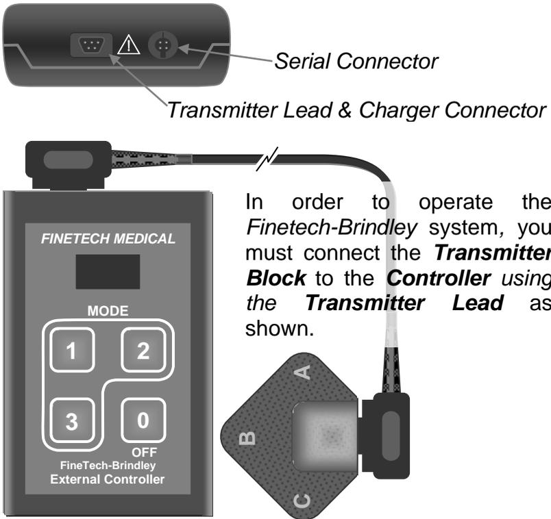
To unplug a connector, always pull the moulded body of the plug in the direction of the arrow as shown and not the lead.
