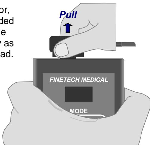
To unplug the connector from the *Transmitter Block*, hold the *Transmitter Block* in one hand and pull the plug with the other hand.
